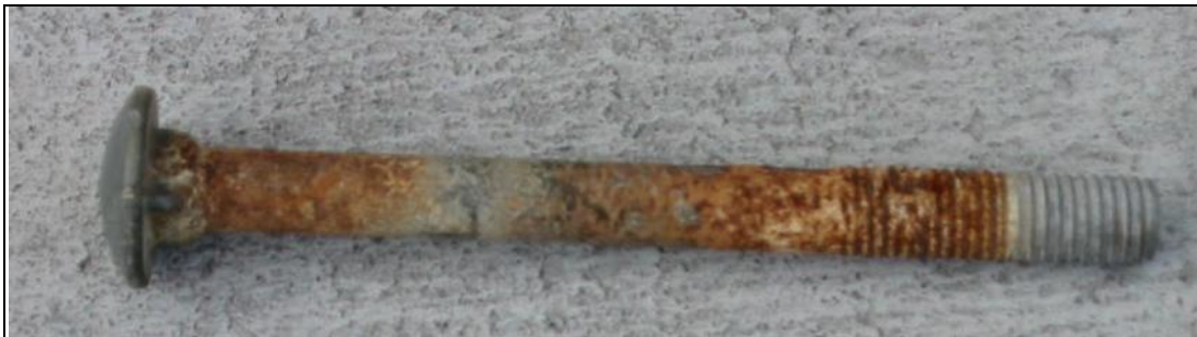
Galvanised bolt after 12 months in spotted gum in Gatton
