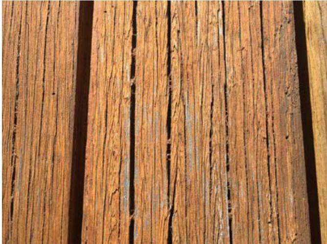
The picture to the left is of 13 year old blackbutt used in a barbecue table in full sun. It is not aging gracefully. When you go away from the timbers that were traditionally used in an application and just go by a durability rating you can get this disappointing result. When writing to one timber merchant in Perth recently about jarrah, he commented *"It's funny you mention Colour, over here lighter wood preforms miserably in our climate,*
