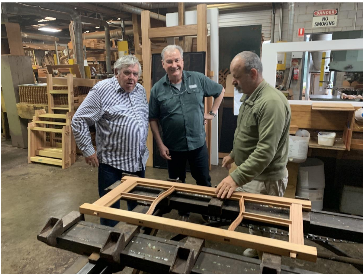
John Coates, an employee and myself inspecting the assembly of a traditional window
