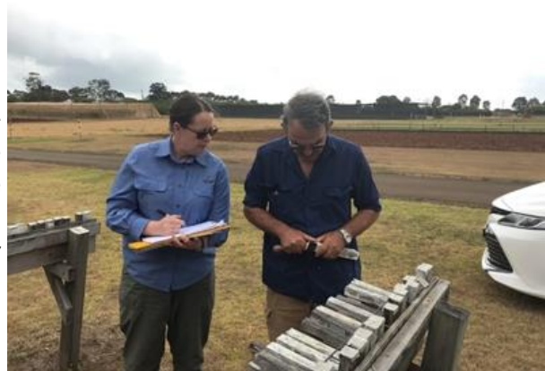
Figure 3. The handheld x-ray fluorescence unit used to evaluate quality of CCA treated timber.
