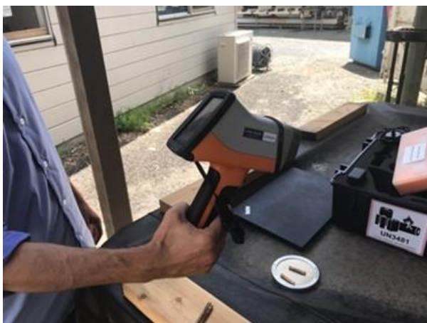
Figure 3. The handheld x-ray fluorescence unit used to evaluate quality of CCA treated timber.
