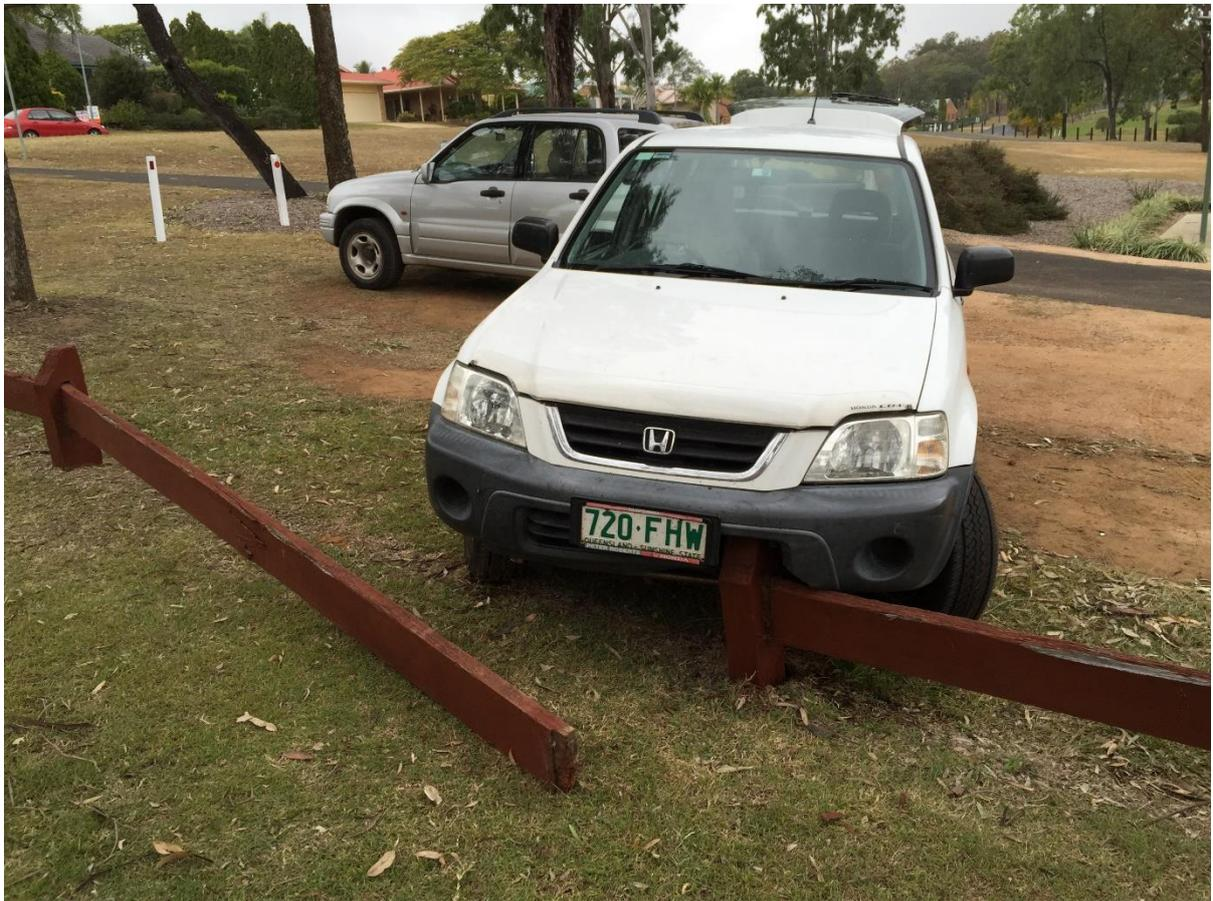
Compare that outcome with these almost 30-year-old traffic barriers I supplied opposite my house. The driver hit the accelerator, not the break (the risk at the above carpark) but the bollard drove the radiator into the motor and stalled the engine. the car was written off with the subframe damage. And it is not designed as a crash barrier!
