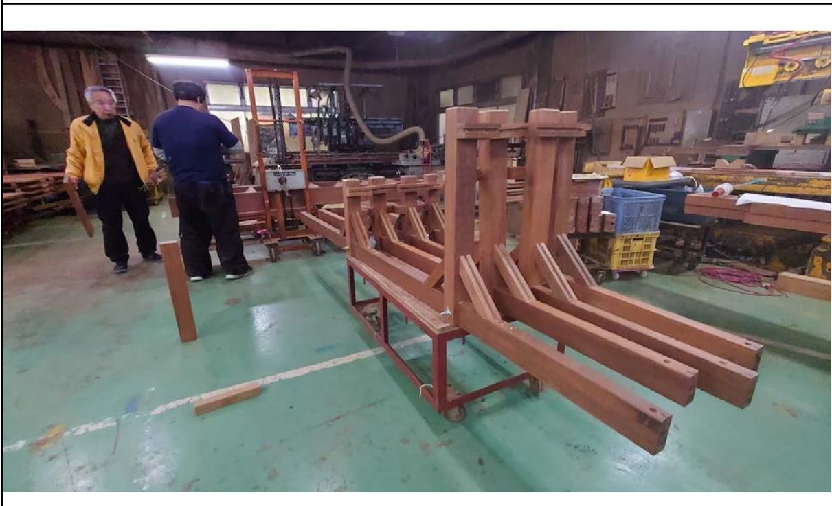
The deck was pre-cut and partially assembled in the factory under a controlled environment and the scrutiny of the Kuratas. They were previously furniture manufacturers and everything is done with that level of precision and quality. The timber quality is similar to that in the first article. Kurata Co order well and their miller knows their expectation.
