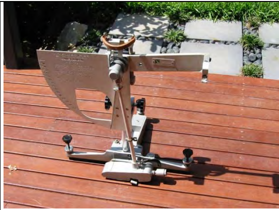
Slip testing a dressed and sealed deck
